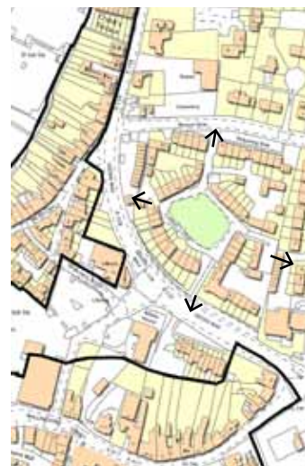
In blocks with only a single shared access point, pedestrian and cycle access should be maximised
