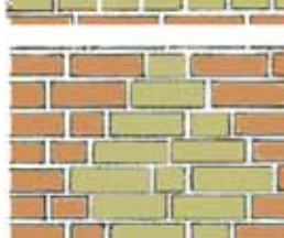
Diaper work of many different patterns ranging from diamonds to crosses and numbers is prominent in different brick colours and sometimes is honeycombed where ventilation is required, such as barns
