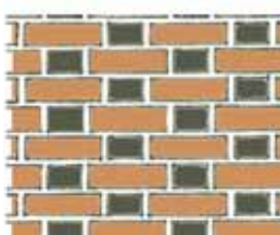
Flemish Bond with blue bricks or flared/ glazed headers is another frequently found alternative especially in Zones 2C and 3. Rarely it is seen with Gault bricks
