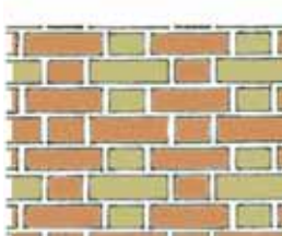
Cross or Flemish: Cross bond is very occasionally seen and only in decorative Victorian properties found in Zone 2c and uses Gault bricks
