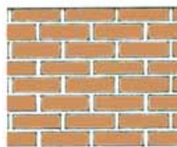
Running or Stretcher Bond: A bond composed of overlapping stretchers. Often found on modern mass produced housing.
