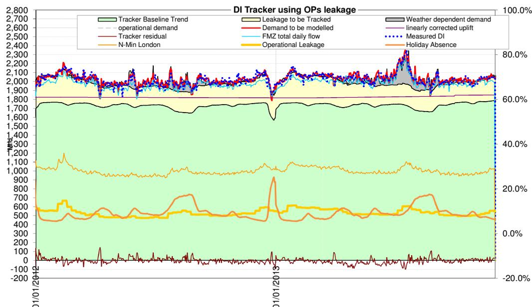
Figure 15: Tracking base demand using a percent empty stat derived from our DWUS panel telemetry
