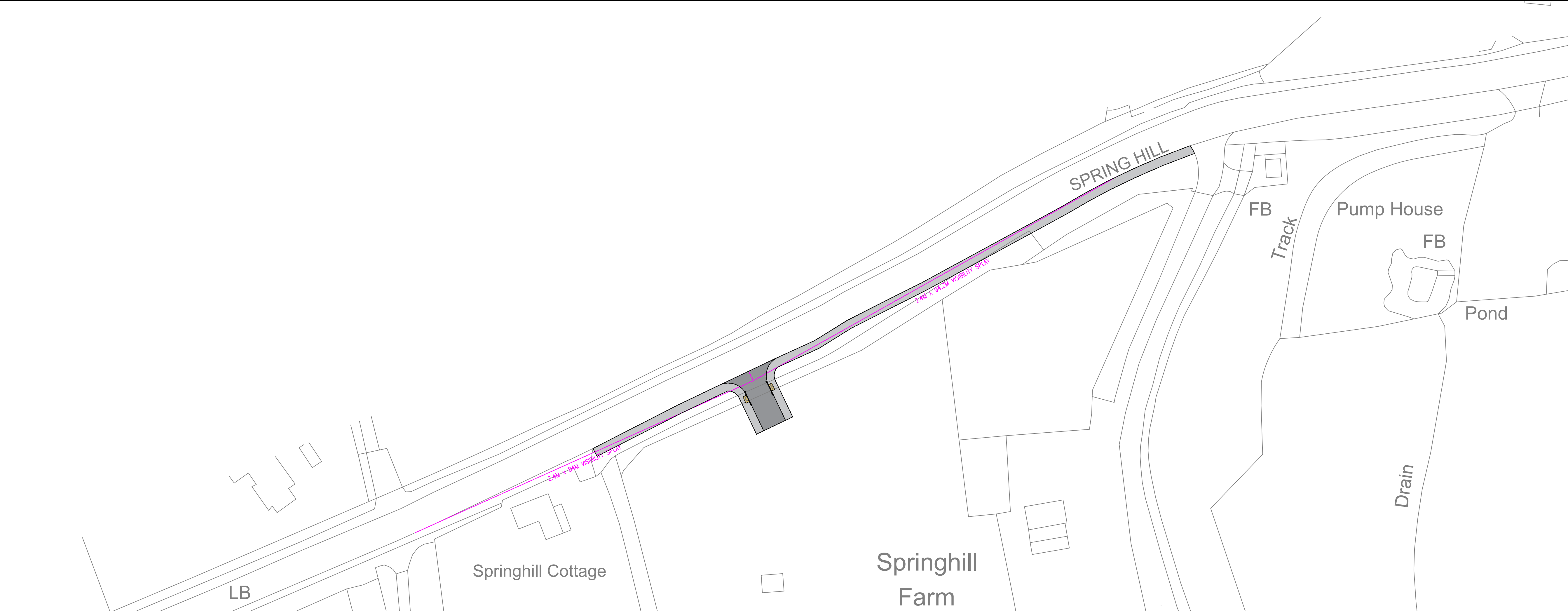
EASTERN SITE ACCESS OPTION – SPEED SURVEY VISIBILITY SPLAY (SCALE 1:500)
