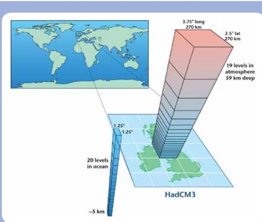
Figure 2.5: The horizontal and vertical structure of the HadCM3 climate model.
