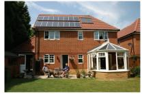
council's preference is for solar collectors to be incorporated into the roof finish at a low level, where they are less likely to be visually prominent. The optimum location is facing slightly west of due south and at a tilt between 30° and 40° although a collector set anywhere between East and West and at a tilt of between 10° and 60° can achieve high levels of performance.
