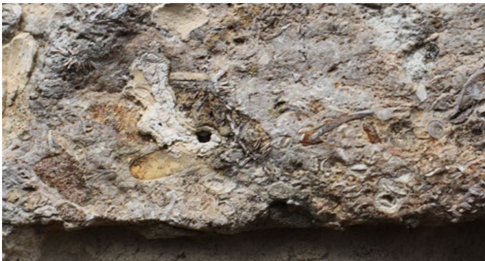
Fig 12. Close up of fossiliferous limestone typical of Stanford, found on Chapel Road
